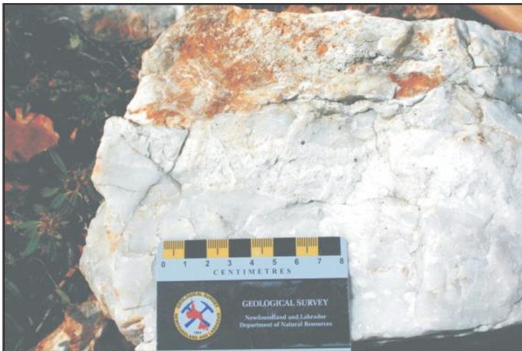
Plate 28: Lattice bladed texture, indicative fluid boiling, hosted within chalcedonic silica vein, Big Easy prospect.
