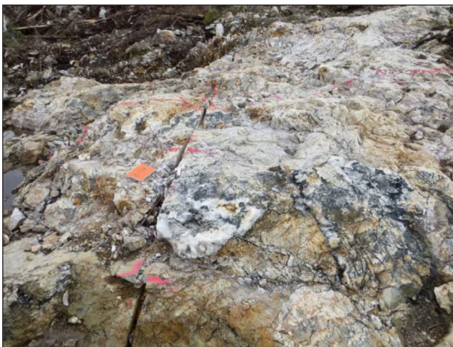
Figure 21. Stockwork quartz–tourmaline–pyrite veins hosted in strongly sericite–silica altered quartz porphyry, Marathon Deposit. Source for the photos: Marathon Gold, 2021.
