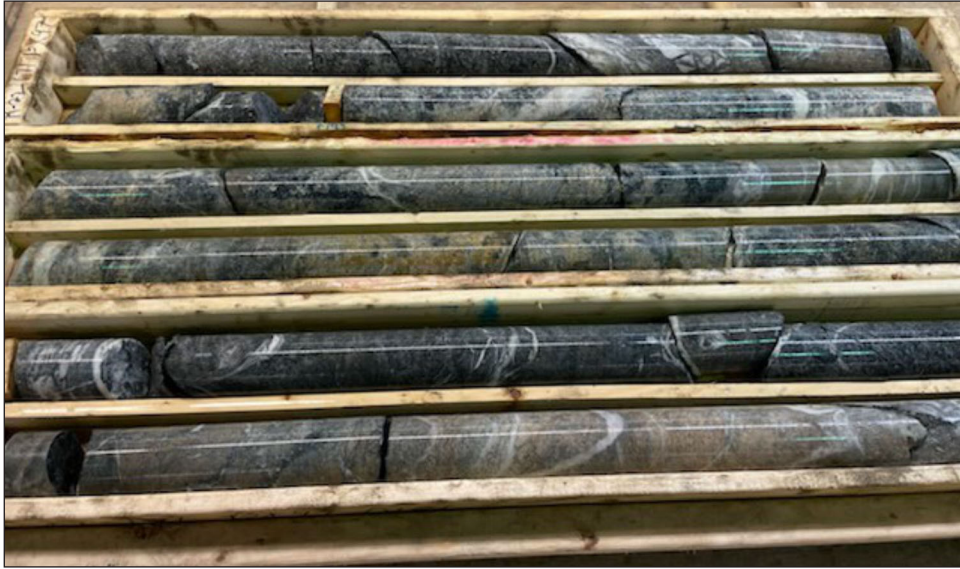
Figure 30. Carbonate and potassic alteration in mineralized gabbro from the Midway Prospect.
