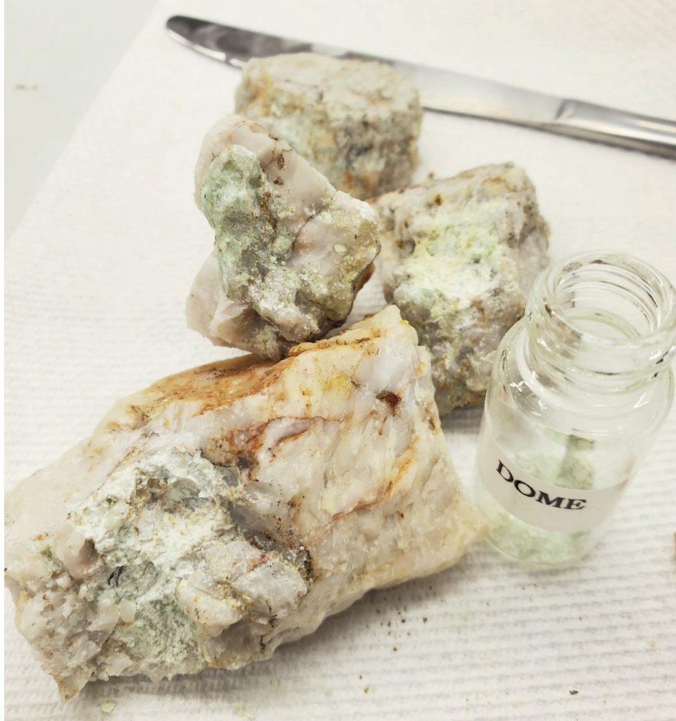
Figure 10. Typical alteration style around gold bearing veins at the Dome Prospect.
