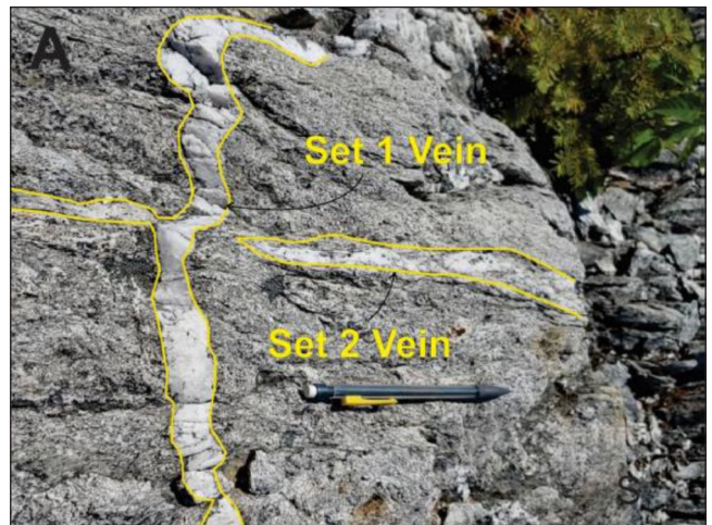
Figure 22. Field relationship between Set 1 (extensional) and Set 2 (shear parallel) veins, Leprechaun Deposit.
